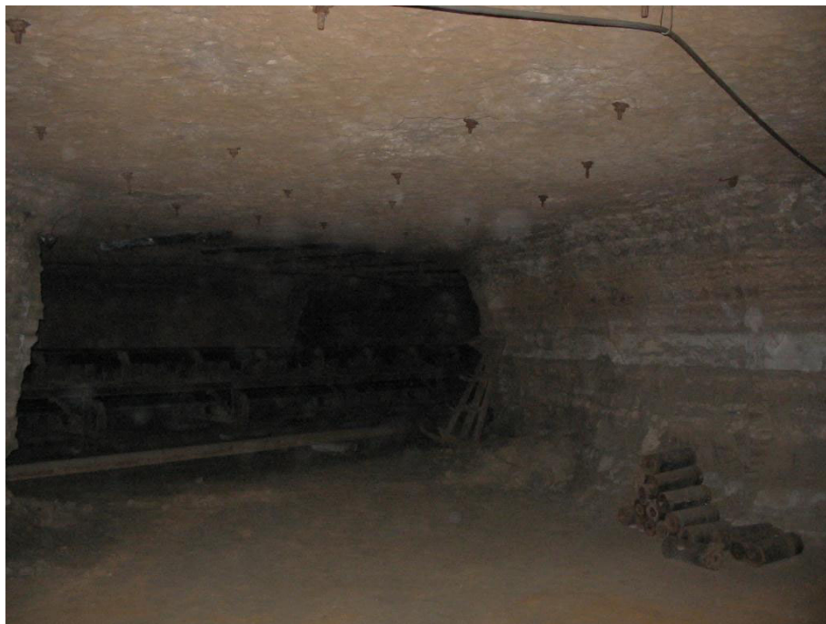
Fig. 6. Room and pillar mining leaves underground free space (Estonia mine) [16].
